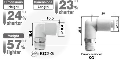
$\ast 1:$  Previous KG series model: Male elbow, applicable tubing O.D. ø6, connection thread R1/8
