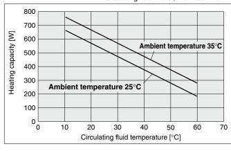
Circulating fluid: Water, Flow rate: 1 L/min, When constant fan speed mode is selected
