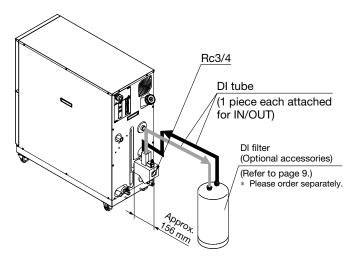
\* Install the DI filter outside the thermo-chiller for piping. Secure the space for installing the DI filter on the rear side of the thermo-chiller. \* It may go outside of the temperature stability range of ±0.1°C when this option is
