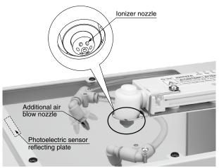
(In addition to the ionizer nozzle, the additional air blow nozzle and photoelectric sensor reflecting plate are installed on the upper surface in the box. Avoid these items being in a collision with a workpiece.)
