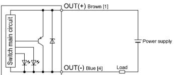
The number shown in brackets [] in the wiring diagram indicates the prewired connector pin number.
